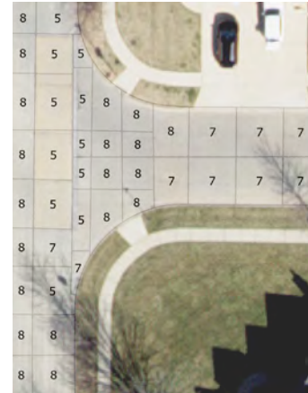
Above is an example of the pavement, slab divisions and ratings displayed via the City's mapping system.
